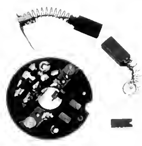
A range of DC motor brushes. The plate assembly consists of permanently mounted phosphor bronze springs with attached contact point. Failure of the motor was due to breaking of a contact point.
